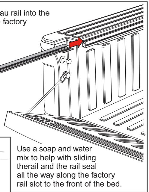
Use a soap and water mix to help with sliding the rail and the rail seal all the way along the factory rail slot to the front of the bed.
