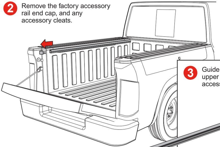
**Steps 2 through 6 are required and repeated on both sides.**
