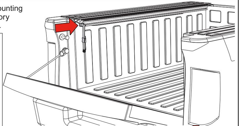
Slide the strap assembly forward towards the cab.
